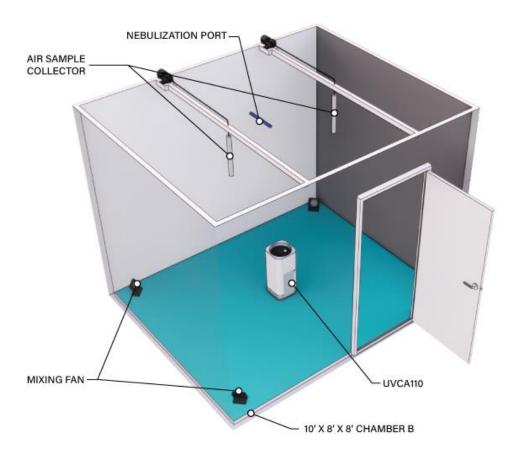
Figure 1. Room layout for control and experimental trial.
