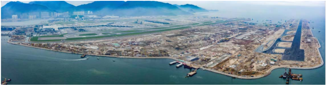
Three-runway System reclamation works / Source: AAHK Third Runway Website
